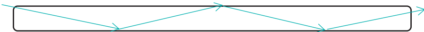
Figure 5.5 A light ray sent into a fiber-optic cable experiences total internal reflection at each encounter with the surface, so the ray emerges from the other end.
